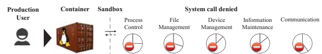
Fig. 1: Our approach in a nutshell. Mining phase monitors accessed system calls when testing. These system calls make up a sandbox for the container, which later prohibits access to system calls not accessed during testing.
